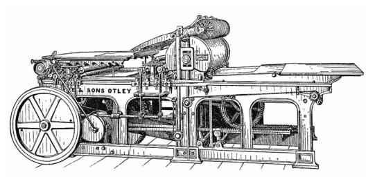
Wharfedale stop cylinder printing machine as used at Murray's
