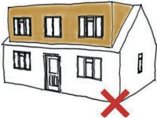
Figure 19 Dormers should be designed so that they fit comfortably within the roof of the building
