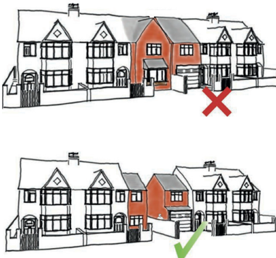
Figure 1 Extensions should be subordinate and positioned so they do not dominate the street scene.
