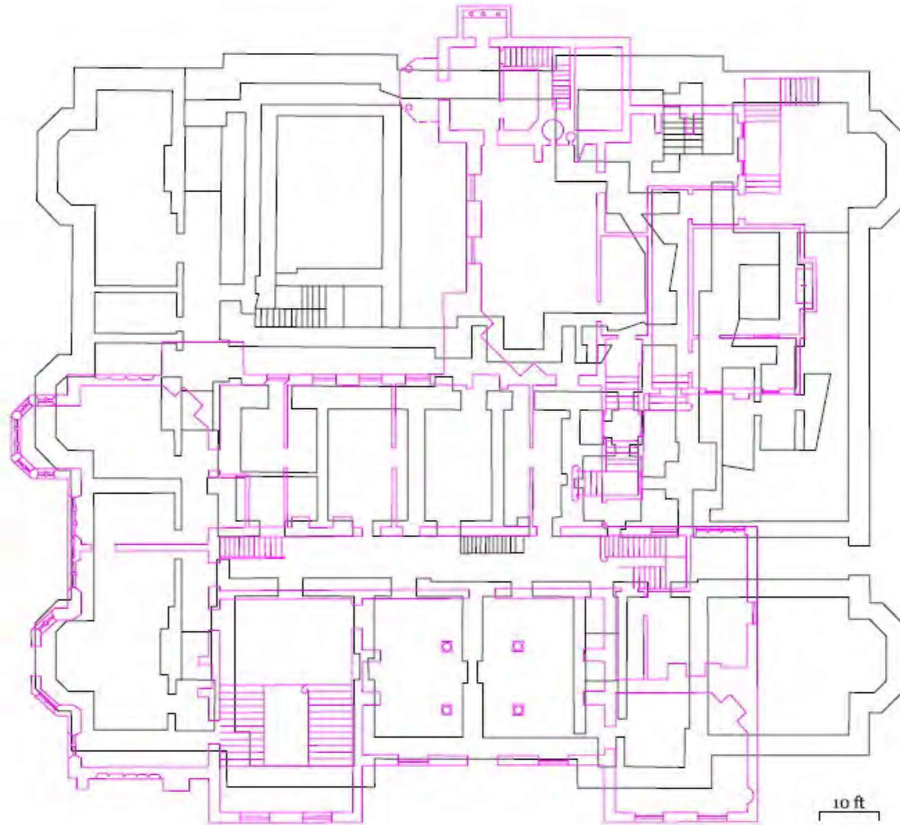
The old Haigh Hall Ground floor plan (pink) overlaid on the current Haigh Hall from unknown author: 2010
