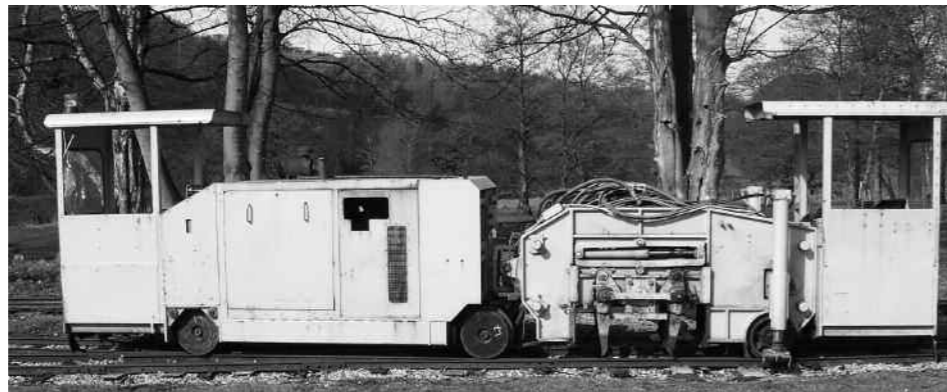
The Gullick Dobson Track Ballaster, painted yellow from its original NCB white and with extended cab roofs, after its use on the Welsh Highland Railway. Photographed, March 2008.
