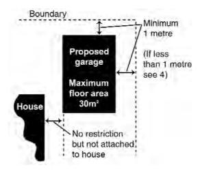
4 If a detached garage is sited less than one metre from the boundary of a property it must be constructed substantially of non-combustible materials and have a floor area not exceeding 30m<sup>2</sup> to be exempt.
